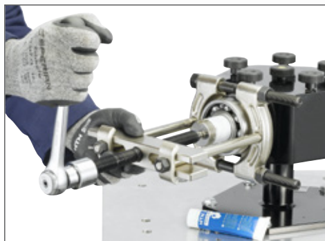
Extraction with separator
